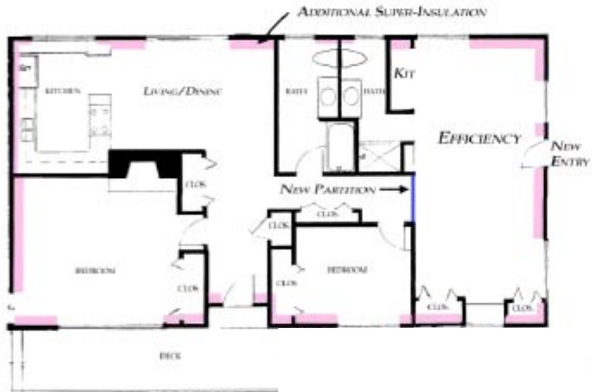
Here a non-bearing partition is removed to make an efficiency, and the old living room partitioned into a bedroom for a two-bedroom unit.
