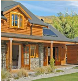
COMPACT, HALF THE SQUARE FOOTAGE, 1-1/2 STORY, SUPER-INSULATED DESIGN REDUCES HEATING LOADS BY 80%
